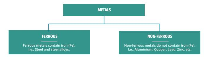
Steel, an iron alloy containing less than 2% of carbon (highly ductile), is by far the most used metal in the world. Followed by aluminium and copper, and other non-ferrous metals such as lead, zinc, nickel, titanium, cobalt, chromium and specialty and precious metals.
